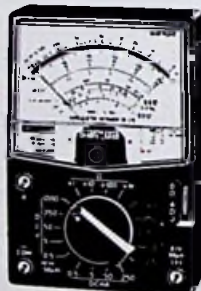
U/50DX. Meetbereiken: DCV, DCA, ACV, Ohm, DB.
